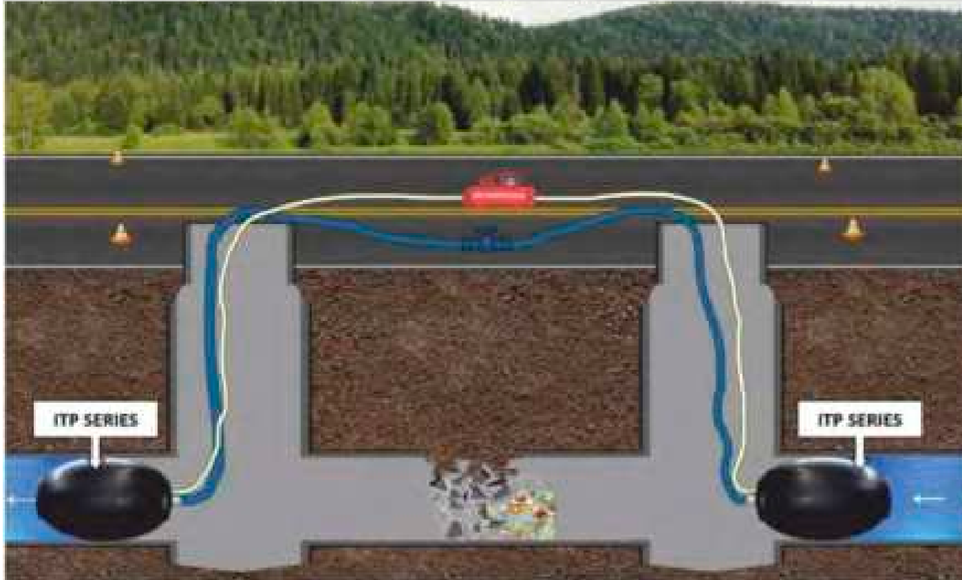
Picture-4 ITP series in pipeline water leak bypassing
